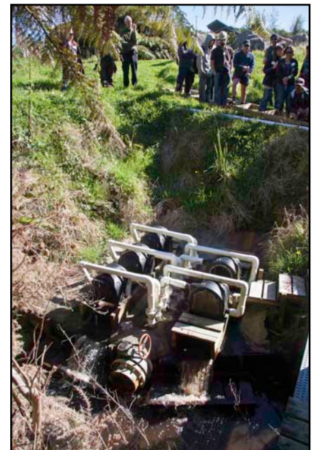
Above: Microhydro turbines turn the waters of the creek into electrical energy.
